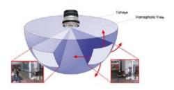
A monitoring centre operator conducting a remote Virtual Patrol or alarm verification on a RemoteGUARD enabled MOBOTIX camera can correct one or more image sections for perspective in the hemispheric view, allowing the operator to monitor several different areas of a room at the same time, something that a mechanical camera is not capable of doing.
